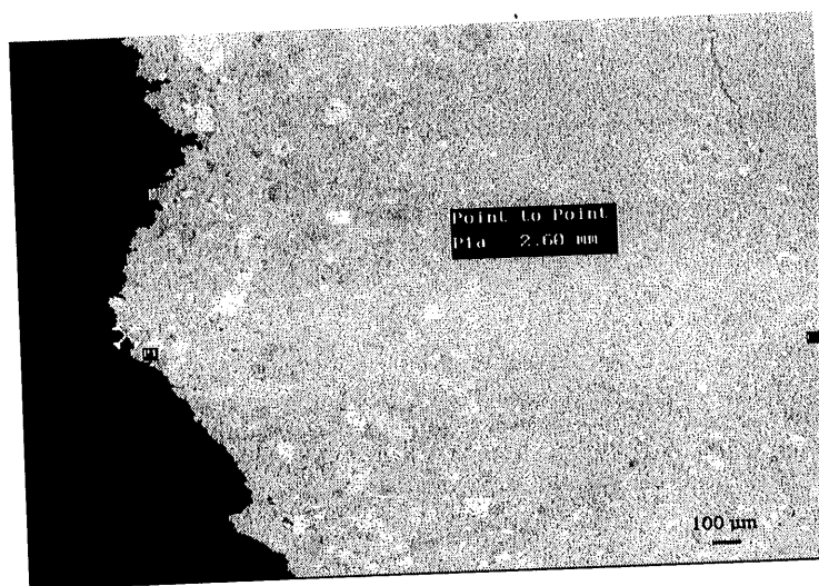
Figure 1. SEM backscatter image of a polished mount representing a portion of a single Bauxsol grain showing the very fine particle mineral constituents.
