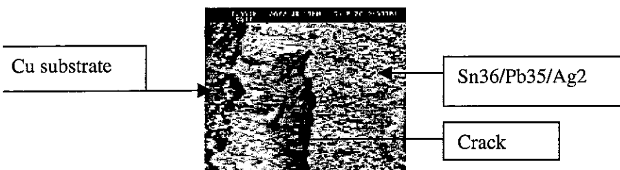
Figure 9. Side view of sample 5 failed at Copper/PCB interface. Opening crack through the solder is shown
