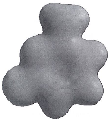
Figure 5: The charge density of cytosine with one H 2 molecule adsorbed on the hexagonal position as calculated from the first principles.
