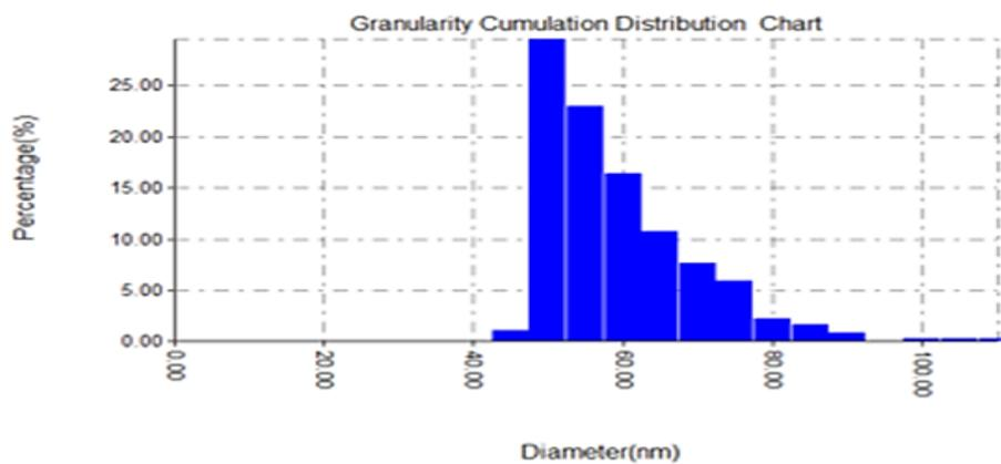
Figure 1. AFM analysis of the purchased ZrO<sub>2</sub> nanoparticles.
