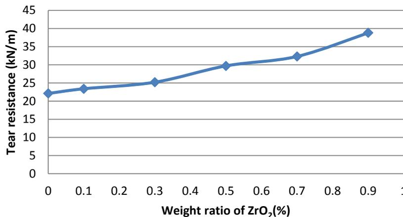
**Figure 4.** Tear resistance of the polymer/ZrO<sub>2</sub> composite as a function of the ZrO<sub>2</sub> weight ratio.
