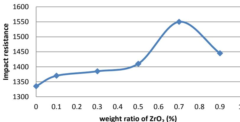
**Figure 6.** Impact resistance of the polymer/ZrO<sub>2</sub> composite as a function of the ZrO<sub>2</sub> weight ratio.
