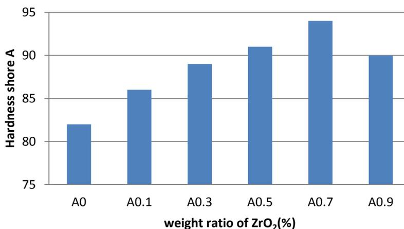
**Figure 5.** Hardness shore A of the polymer/ZrO<sub>2</sub> composite as a function of the ZrO<sub>2</sub> weight ratio.
