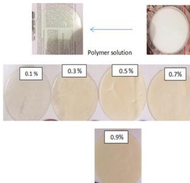
**Figure 3.** Optical images of the polymer-ZrO<sub>2</sub> composites as a function of the ZrO<sub>2</sub> weight ratio.
