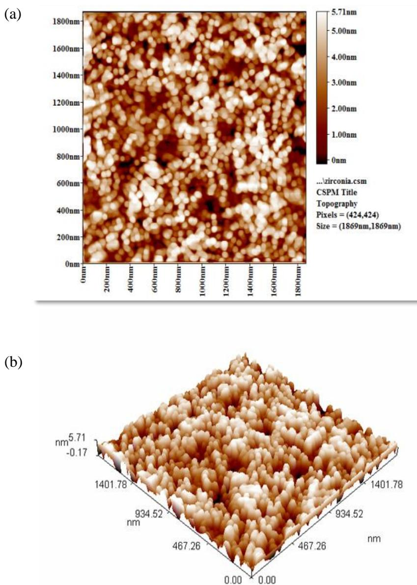
Figure 2. Plots show (a) two- and (b) three-dimensional AFM presentation of ZrO<sub>2</sub>.
