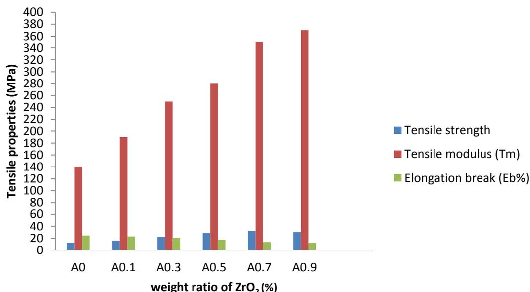
**Figure 7.** The tensile properties of the polymer/ZrO<sub>2</sub> composite as a function of the ZrO<sub>2</sub> weight ratio.
