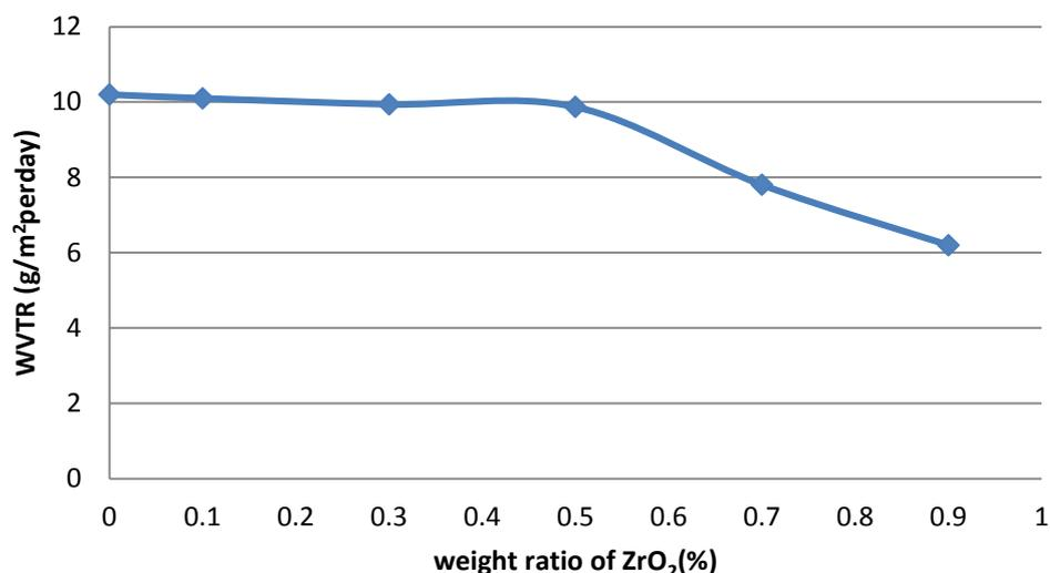
**Figure 8.** Water vapor transmission rate of the polymer/ZrO<sub>2</sub> composite as a function of the ZrO<sub>2</sub> weight ratio.
