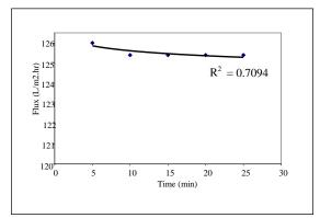
Figure 1 Flux versus time for 100 kDa PES membrane
