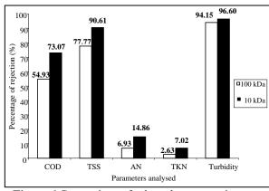
Figure 6 Comparison of selected parameter's rejection performance between 100 kDa and 10 kDa PES membrane
