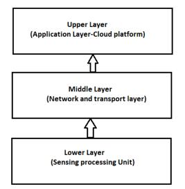
Figure 1. Three layer architecture of IoT
