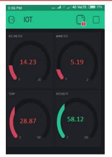
Figure 4.(d) Acquired PV parameters at 3:06 PM
