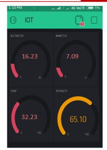
Figure 4.(b) Acquired PV parameters at 1:10 PM
