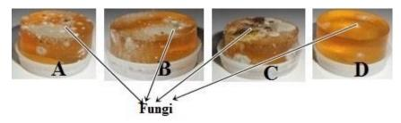
Figure 4. Durability Test Results of Gelatin-glycerin Samples at 27°C
