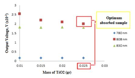
**Figure 9.** Relationship between transmitted intensity of laser after passing samples as a function mass of TiO<sub>2</sub>
