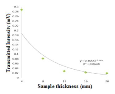
**Figure 10**. Relationship between transmitted intensity of laser after passing samples as a function sample thickness.
