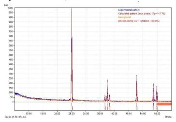
Fig 1. Diffractogram of TiO<sub>2</sub>
