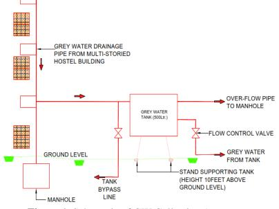
Figure 1. Schematic of GW Collection Arrangement
