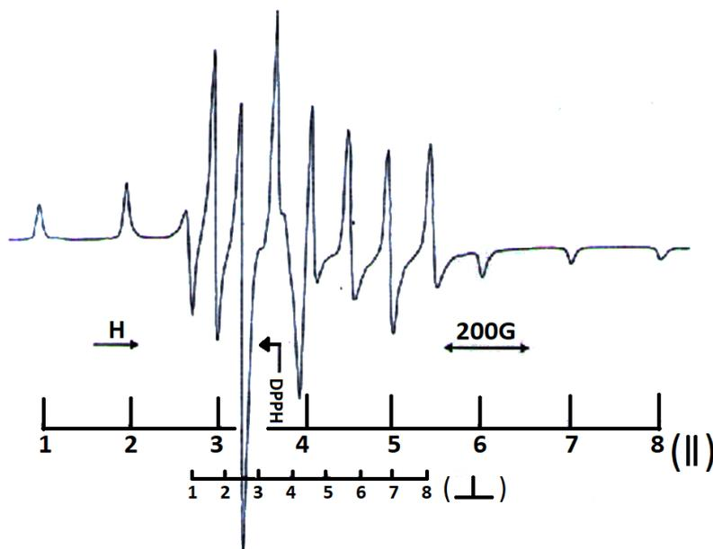
Fig.2 EPR of vanadyl doped  $Zn_{0.25}Mg_{0.75}(NH_4)_2(SO_4)_2 \cdot 6H_2O$  [H(DPPH)= 3385G]. Parallel and perpendicular hyperfine groups are marked by vertical lines below the spectrum.
