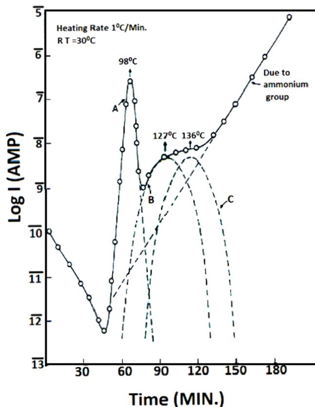
Fig.3 Temperature variation for current vs. time for zinc ammonium sulphate hexahydrate pellet. The composite peak at 131°C is shown as deconvoluted into curves 'B' and 'C'
