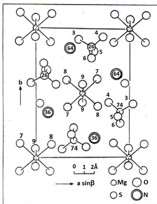
Fig.1 Crystal Structure of MASH. The number at the sulphur and nitrogen items indicate their Z-Coordinates
